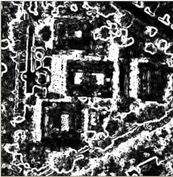
Fig. 6: Shadow Boundaries Resulted from applying Uniform Filter on the Third Channel (C3)
